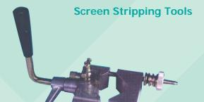
> Removes bonded semi-conductor screen
