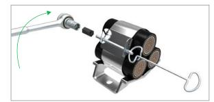
Pull slack into outer loop. Insert split pin from right hand side around outer layer of strap about 10mm from end. Push plastic shear torque adaptor fully onto the end of the split pin and attach 13mm socket wrench. To tension the strap rotate key anti-clockwise with the socket wrench
