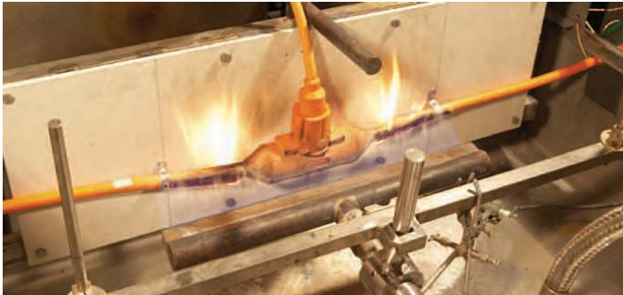
BS6387 Category Z - Resistance to fire with mechanical shock; 950°C for 15 minutes with 30 second hammer blows.
