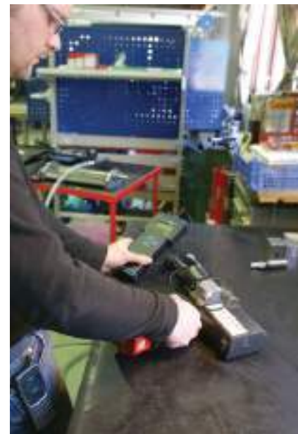
Elpress service department, calibration of crimp tool PVL1300.
