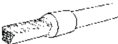
Crimped pre-insulated end terminal.
