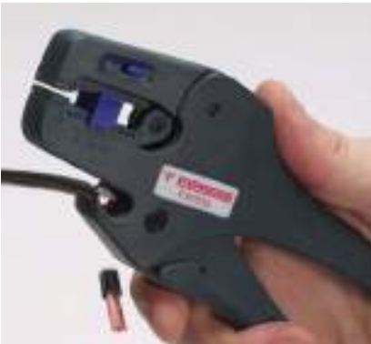
EMBLA, ergonomically designed cutting- and stripping tool.
