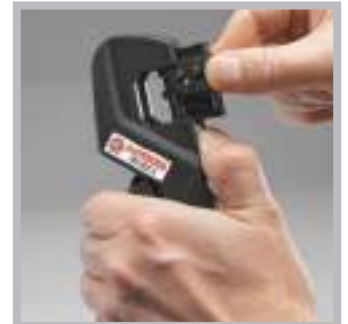
OMP11 For crimping of modular- plug RJ11.
