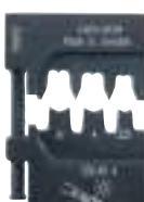
OMS4 For crimping of solar connectors Ø 4 mm, with open barrel conductor crimp 2.5 - 6.0 mm 2 .
