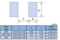
In order to expect the self alignment effect, it is recommended that land width is almost the same size as terminal of capacitor, and space between lands (c) nearly equal to the space between terminals for appropriate soldering.
