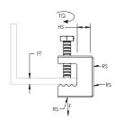
Material: Spring Steel Finish: nVent CADDY Armour
