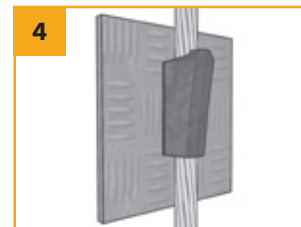
VERTICAL CABLE TO VERTICAL METALLIC SURFACE
