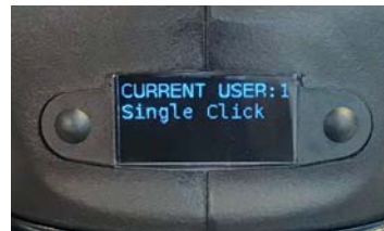
Safety Function: ** adjustable crimping operation start with optional one or two 'click' trigger for safer handling of the tool.
