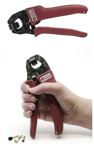
PEB0110T18 is a new tool for crimping end sleeves that are up to 18 mm long in a single crimp. The crimp tool is self-adjusting, thus ensuring quality. Front feed makes the tool user-friendly and convenient in confined applications. The crimping tool is tested for 50,000 crimps without calibration and is thereby "life-time-calibrated".
