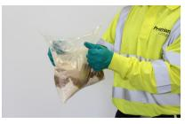
5. Make sure that the membrane seal is completely open before mixing the powder and liquid together.
