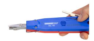
With the Sensor No. 40, wires with a conductor diameter of 0.35 - 0.9 mm and a wire diameter of 0.7 - 2.6 mm can be wired into LSA panels or blocks. With a gentle push on the tool, the wires are inserted and cut off in just one single step. Manual stripping or screwing is not required.
