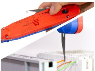
Note Working with WEICON Stripping Tools is only permitted on zero-potential, non-current-carrying cables and conductors.
