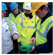
Measuring earthing resistance of the earth connection
