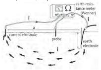
Measuring earthing resistance of the earth connection - Method 1
