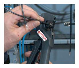
Professional contact crimping tool with interchangeable dies for the installer or service technician.
