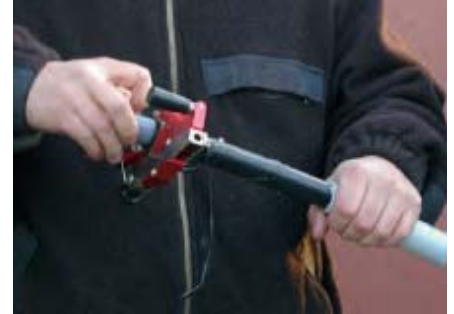
Stable FBS1722 stripping tool delivers better and smoother results than most other stripping tools.
