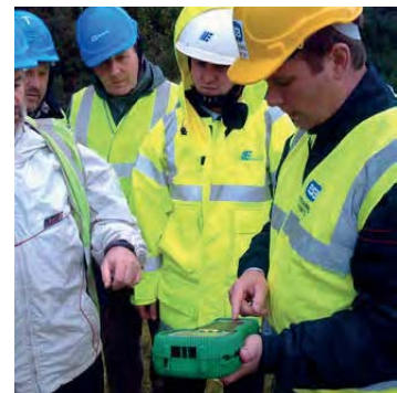
Measuring earthing resistance of the earth connection
