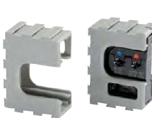
OSW0360 Crimping die for Elpress MOBILE tool for crimping through connectors with heat shrink insulation 0.3-0.75 mm 2 and 4-6 mm 2 . AWG 11-9.
