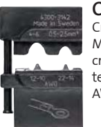
OKB0725 Crimping die for Elpress MOBILE tool for punch crimping uninsulated terminals 0.75-2.5 mm 2 . AWG 18-13.
