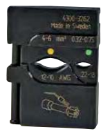
OSW0360 Crimping die for Elpress MOBILE tool for crimping through connectors with heat shrink insulation 0.3-0.75 mm 2 and 4-6 mm 2 . AWG 11-9.
