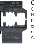
OEB1625 Crimping die for Elpress MOBILE tool for crimping end sleeves 16-25 mm 2 . AWG 5-3.
