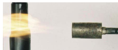
Shrinkage of the insulation is achieved by using heat.
