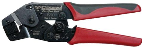
Tested and certified mechanical hand tool for crimping end terminals 0.5-6 mm<sup>2</sup> and insulated TWIN end terminals 2 x 0.5-2 x 4 mm<sup>2</sup>.
