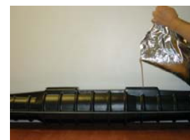
Pouring of polyurethane resin
