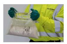
3. To start the mixing process, hold the bag as shown above, so that the liquid is forced onto the powder.
