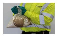
4. Squeeze the liquid through the membrane seal and onto the powder.
