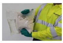
2. Aerate the powder by gripping the pouch at each end and tumbling the powder for up to thirty seconds, this will facilitate mixing.
