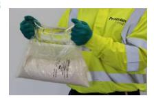
3. To start the mixing process, hold the bag as shown above, so that the liquid is forced onto the powder.
