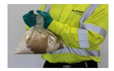
4. Squeeze the liquid through the membrane seal and onto the powder.
