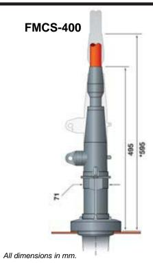
\*Minimum dimensions necessary to disconnect.
