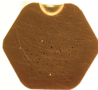
Cross section of DUAL crimp
