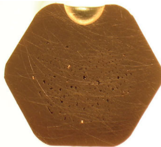
Cross section of DUAL crimp
