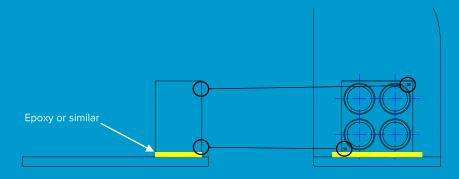
2 Set a frame, to sandwich the Bell Block. Ensure the frame is flush with the Bell Block and that there are no gaps. If necessary mask off the female connectors on the Bell Block to stop dirt/debris or concrete entering the connectors. Ensure the bell block does not move during concrete curing.
