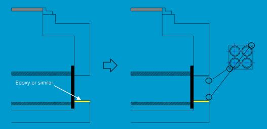
Fill the gap above the Bell Block with epoxy putty or similar. It may be necessary to use a space to fill the gap if too large. Ensure that the bell block connectors are free from putty to ensure a secure connection to EFLEX Square. If a watertight seal is required apply epoxy putty or similar around the edge of the Bell Block on both the inside and the outside of the chamber. Masking tape can be used to prevent concrete entering the bell block connectors.
