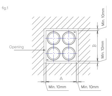
2 Cover the single opening on the inside of the chamber with a plate or similar and hold it in place with a wooden block/spacer or similar, while work is carried out.
