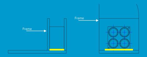
Pour concrete into the frame and ensure there are no leaks. When cured, remove the frame. If a watertight seal is required, apply epoxy putty or similar around the edge of the Bell Block on both the inside and outside of the construction (highlighted yellow)
