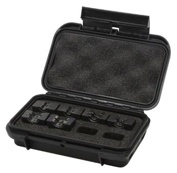
A complete kit with crimp dies for hexagonal crimping of 10-70 mm<sup>2</sup> using Elpress 350 Mini system, supplied in a waterproof and impact resistant box. The box contains six crimp dies that cover crimping of Elpress KR/KS and KRF/KSF (standard copper terminals) from 10 up to 70 mm<sup>2</sup>. Additionally, in the box, there are two more empty slots for extra crimp dies of your own choice, for example, for CUT or C sleeves.
