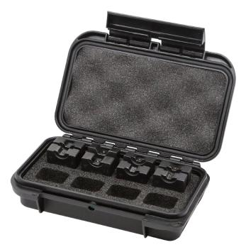
A complete kit with crimp dies for hexagonal crimping of 10-95 mm² using Elpress 600 system, supplied in a waterproof and impact resistant box. The box contains four crimp dies that cover crimping of Elpress KR/KS and KRF/KSF (standard copper terminals) from 10 up to 95 mm² as well as KRX/KSX 10 mm². Additionally, in the box, there are four more empty slots for extra crimp dies of your own choice, for example, for larger sizes or C sleeves.
