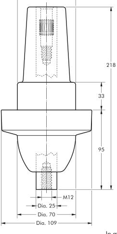
6/10 (12) kV 6.35/11 (12) kV 8.7/15 (17.5) kV 12/20 (24) kV 12.7/22 (24) kV
