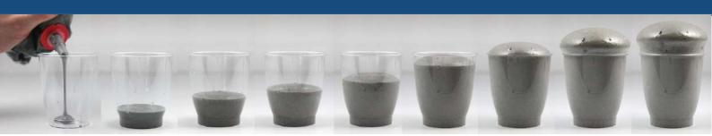
Filoform duct seals type MD are based on a specially formulated two-component expanding polyurethane resin. The polyurethane sealant is packed in a transparent plastic bag with a screw ring. In this plastic bag, the two components are separated by a clamping profile. After removal of the clamping profile, the two components are simply mixed together for 30 seconds.
