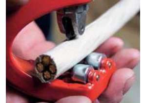
STEP 5: LONGITUDINAL CUT AND REMOVAL OF SECONDARY SHEATH
