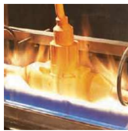
BS6387 Category W - Resistance to fire and water; 650°C for 15 minutes, then for 15 minutes with fire and water
