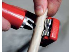
STEP 4: ROTARY CUT ON INNER SHEATH
