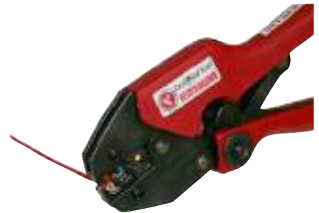
Crimping of Elpress pre-insulated ring terminal with hand tool GSA0760.
