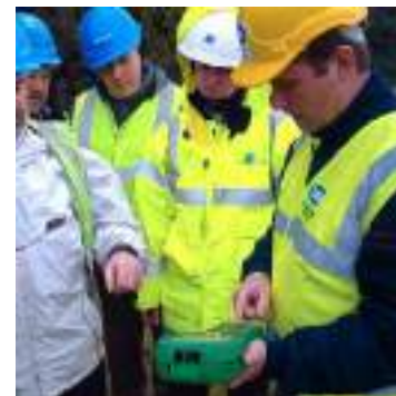
Measuring earthing resistance of the earth connection
