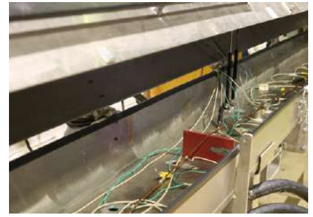
Tests according to IEC 61238-1-1 in own premises.
