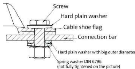
Bolt joint with spring washer.
