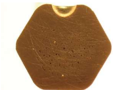
Cross section of DUAL crimp
