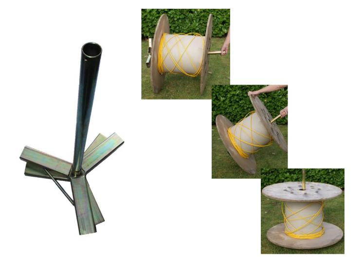
For ease of loading a drum onto the DD1 drum dispenser, a simple yet effective extender can be purchased as an option, it allows you to locate the spigot in the drum centre whilst the drum is in its vertical position. A further advantage is that it allows multiple drums to be stacked safely
