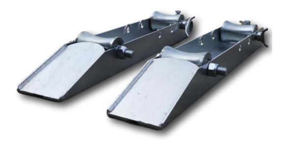
The DR4 medium duty cable drum rotator is suitable for a range of drum diameters up to 1200mm. Drums are simply rolled up the ramp onto the adjustable rollers to allow it to spin freely
