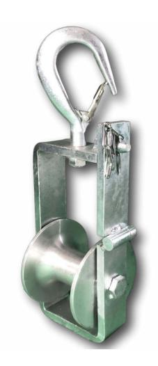
The HR2 hanging roller enables cable to be suspended and winched into position prior to fixing on to tray or cable racking. Fitted with a handy safety hook, the HR2 is quick and easy to install without the need for tools or shackles and is fitted with an aluminium deep diablo roller for effective cable management. The cable roller is suitable for cables up to 75mm diameter with a weight capacity of 100Kg
