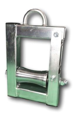
The HR3 hanging roller enables cable to be suspended and winched into position prior to fixing on to tray or cable racking. Similar to the HR1 but fitted with a solid steel roller and heavy duty hook, normally used on heavy cable applications or on the initial roller when lifted from floor to cable rack. The cable roller is suitable for cables up to 120mm diameter with a weight capacity of 150Kg
