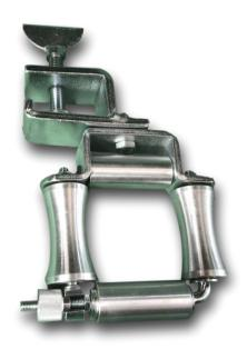
The HR4 clamping roller can be clamped without tools to beams, trays or racks. Also by removing the clamp part it can be bolted directly down to unistrut or trays etc. Fitted with a hinged gate and knurled nut, cable can easily be extracted. The cable roller is suitable for cables up to 60mm diameter with a weight capacity of 100Kg
