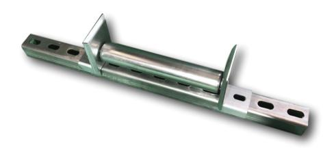
The HR5 unistrut roller can be bolted directly down onto 42mm unistrut (as illustrated), flat plate or square box section up to 40mm. The roller can be made to any width but as standard comes with a 240mm wide roller (340mm overall)
