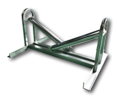
The LR3 V style cable roller is the widest and heaviest duty of the 3 V rollers in our standard range. The V style cable roller leads the cable from the drum into the trench, the design is such that cable is centralised prior to it being fed into the trench. This roller also doubles up as a heavy duty straight line roller or pipe roller and can be positioned in the trench itself. Any width or capacity of V roller can be made on request
