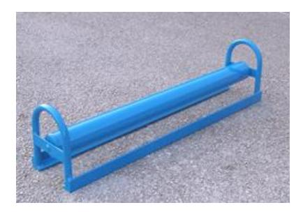
The LR4 cable roller leads the cable from the drum into the trench, the design is such that cable is supported over the full drum width prior to it being fed into the trench. When cables are being laid simultaneously the LR4 can be used as a straight line roller. Any width or capacity of V roller can be made on request
