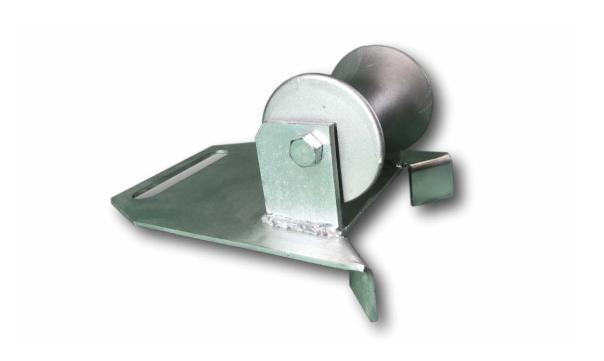
The MR2 manhole cable roller leads the cable from the drum into the jointbox/manhole or the winch bond out of the manhole. The roller has 2 angled hooks for location on the manhole edge or on a 90 degree corner
