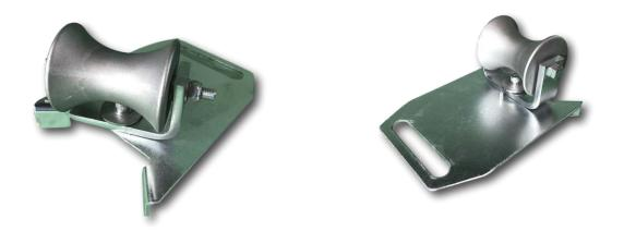
The MR3 manhole cable roller leads the cable from the drum into the jointbox/manhole or the winch bond out of the manhole. The roller has 2 angled hooks for location on the manhole edge or on a 90 degree corner. The unit is similar to the MR2 but the roller section swivels to suit the direction of the pull
