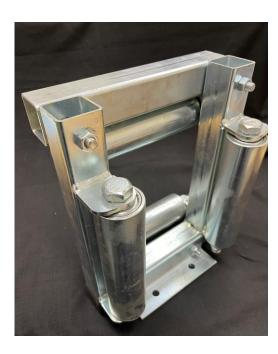
The QR1 quadrant roller can be bolted to floors, beams, trays, racks or fitted to a free-standing frame. Fitted with a hinged/removable gate, cable can easily be extracted. The cable roller is suitable for cables up to 160mm diameter (aperture 170mm) with a weight capacity of 400Kg
