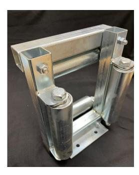
The QR2 quadrant roller can be bolted to floors, beams, trays, racks or fitted to a free-standing frame. Fitted with a hinged/removable gate, cable can easily be extracted. The cable roller is suitable for cables up to 160mm diameter (aperture 170mm) with a weight capacity of 200Kg.
