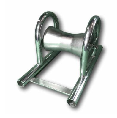
The SLR11 is a heavy duty cable roller for use in most cable laying applications. Very similar to the SLR4 but with an extended base length of 400mm with cross flats set at 300mm for ladder rack applications
