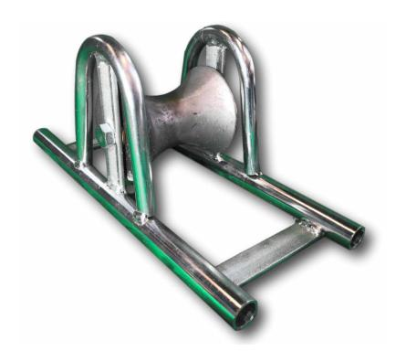
The SLR1E is a compact cable roller for use in narrow trenches and confined spaces, the 'E' version has an extended 350mm long base and cross flats set at 300mm for use on ladder racks
