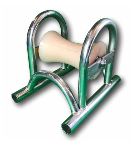
The SLR5P is a heavy duty bridge style cable roller for use in most cable laying applications. The diablo roller is nylon so non-conductive and reduces the risk of damage to the cable
