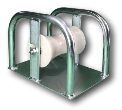
The SLR9P is a heavy duty straight line cable roller for use in most cable laying applications and specifically where the ground is unstable. The base can be drilled as an option for fixing down. The diablo roller is nylon so non-conductive and reduces the risk of damage to the cable
